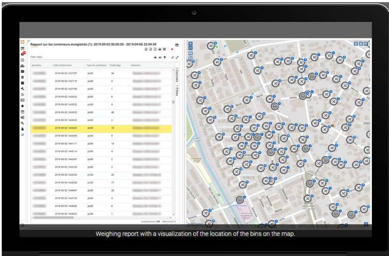
Figure 2. Spatial dashboard provided in relation to on-board weighing solution. (ELTE Group, 2021)
